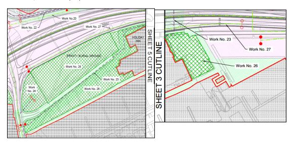
Areas hatched pale green on the Works Plans are proposed to be used for minor utilities diversions and other 'minor' works. Areas cross-hatched green <u>and</u> shaded pale green on the Works Plans are proposed to be used as a work area <u>and</u> for minor utilities diversions and other 'minor' works. Purple dashed line denote proposed utilities diversion works.
